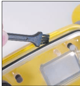
Clean off O-ring with brush provided.
