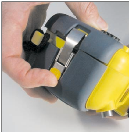
Digital: Push finger into rubber cover and lift latch
