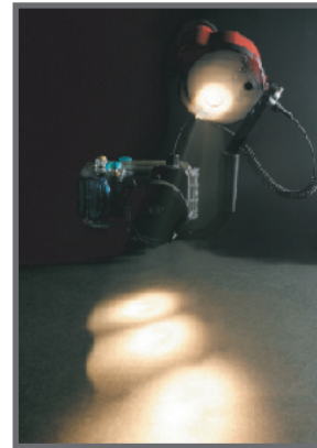
Simple strobe positioning depending on distance to subject by swinging D-2000 on the arm. That's it. You can check if the axis of strobe situate in right position with Focus Light. Focus light never expose on image since it automatically turns off during exposure.
