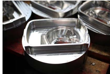
**Your Hugyfot Vision Xs housing is machined from a solid block of marine grade aluminum.**
