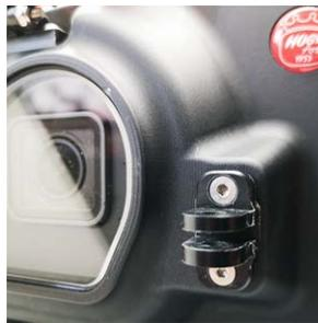
Mount the hinge of the easy flip lens holder to the right of housing flat port using two M3 Allen hex screws (provided with easy flip lens holder). Keep hinge straight edge to the left and curved edge to the right.
